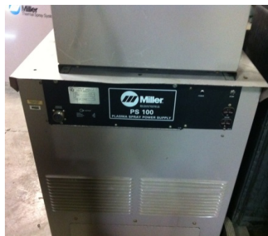
Miller PS 100 Power Supply, 100KW
