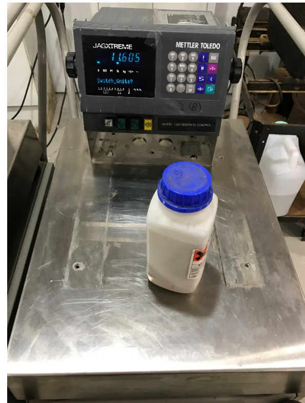
Scale #2 before and after 11kg (11 pounds of powder plus weight of bottle)
