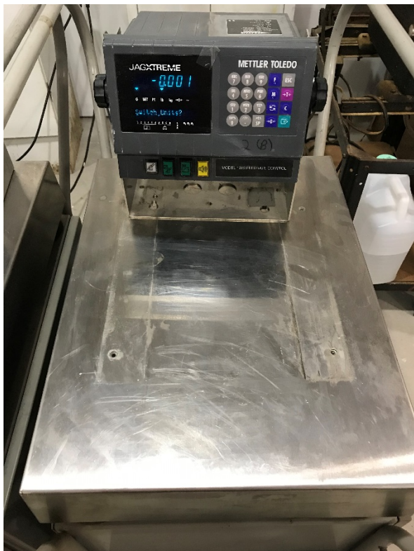
Scale #2 before and after 11kg (11 pounds of powder plus weight of bottle)
