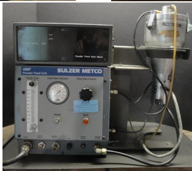
7MC System - 7MC console, 7MR power supply, 4MP powder feeder
