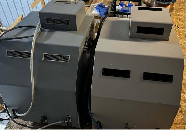
Two Struers Abramin polishers for parts. One of the two does power up and operate, but the down pressure cylinders are weak.
